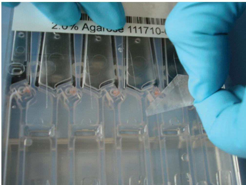
7. Pipette your samples out of the elution module as usual. If the modules are properly sealed, the final elution volumes will be within 1-2 ul of the starting values.
