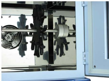
**Step 2** On the left side, align the rotisserie notch with the pin, and release
