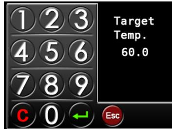
*\*Note: The calibration value varies accordingly to Users' preference. The input value should be the temperature where you control your experiment at most frequently.*
