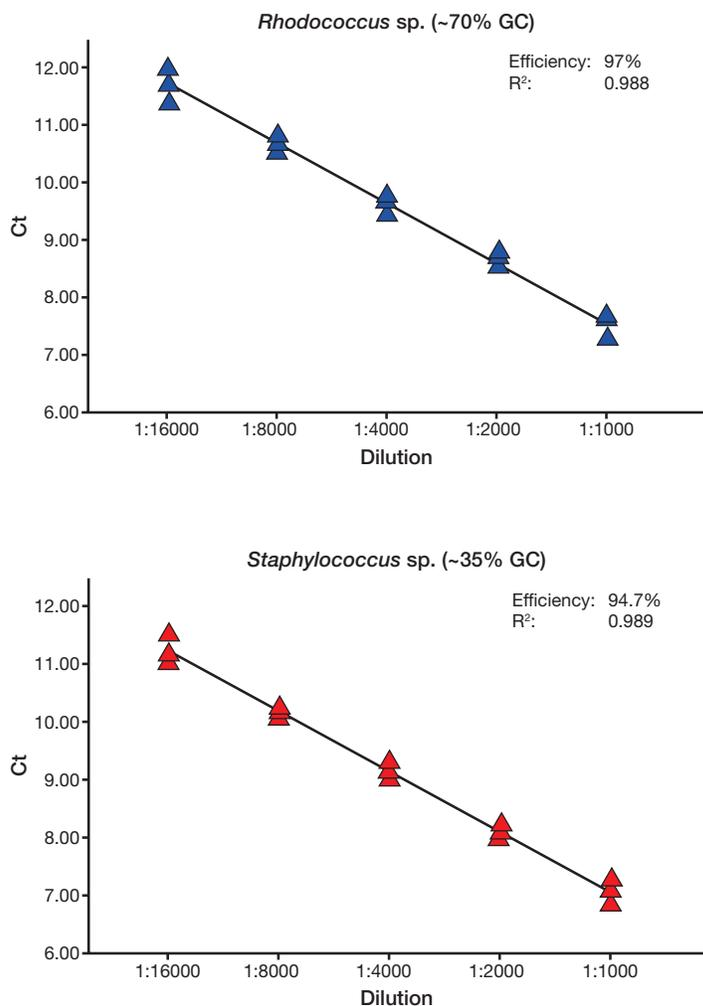
**Fig 6. Amplification efficiency of libraries with a high and low-GC content.** Two-fold dilution series (1:1000 through 1:16000) were prepared in triplicate, and qPCR performed according to the recommendations in the product technical data sheet.
