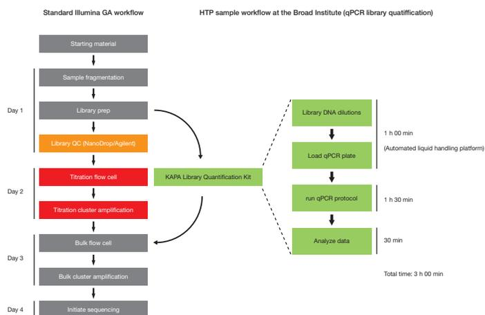
**Fig 2. Streamlined workflow using qPCR library quantification.** Performing the assay in a 384-well format allows for 96 samples to be processed along with DNA Quantification Standards in a single run. qPCR set-up time using the Bravo Automated Liquid Handler is approximately 1 hour. This, combined with a 1.5 hour qPCR assay, enables approximately 500 samples to be quantified by 1 full-time employee per day.
