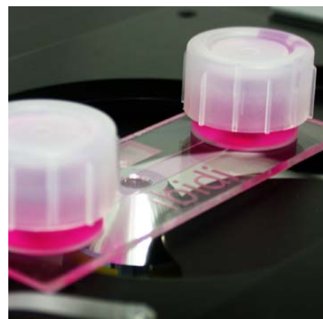
The \mu -Slide I mounted on a microscopic stage.
